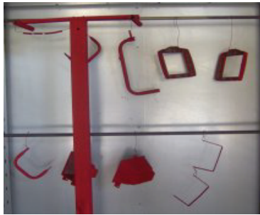
Coated parts hanging in oven to be cured
